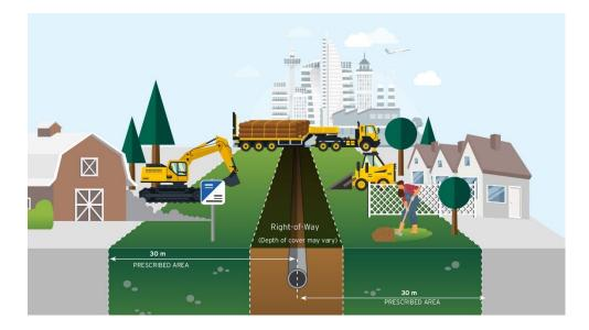
\*As per the CER regulations, all activity within the Prescribed Area which is the area of land that extends 30 meters perpendicularly in both directions from the centerline of the pipe, as described in the representation above, requires written approval from the pipeline company. This work includes but is not limited to vehicle or mobile equipment crossing (outside a travelled or public road); construction, on, along or under a pipeline; or any ground disturbance activity.
